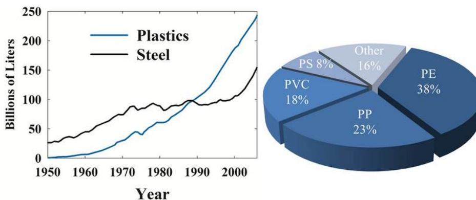
**FIG. 2:** History of global plastics versus steel production and 2007 market share of global thermoplastics production. (A) In 1989 the production of plastics by volume exceeded that of steel. (B) Thermoplastics global market share, highlighting the four most common polymers: polyethylene (PE), polypropylene (PP), polyvinylchloride (PVC), and polystyrene (PS).
