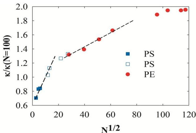
**FIG. 5:** Thermal conductivity of PS and molten PE versus the average number of monomers in each chain  $N$  (proportional to the MW). The thermal conductivity increases with the square root of the chain length at moderate chain lengths and eventually converges to a constant value.
