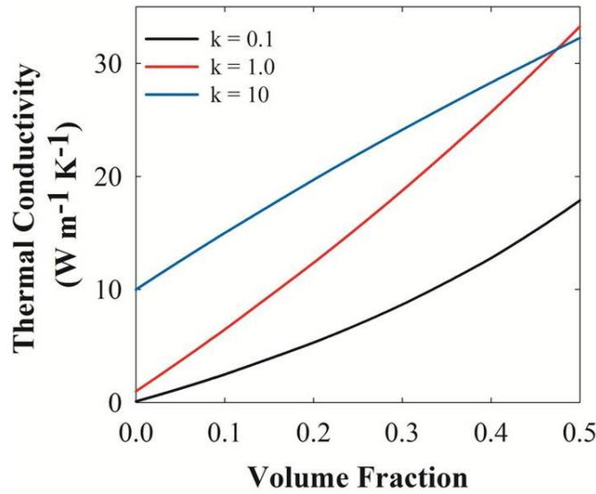
**FIG. 6:** Graphite nanoplatelet–polymer composite thermal conductivity model predictions. This calculation assumes the thermal interface resistance between the platelets and polymer matrix is  $10^{-8} \text{ m}^2 \cdot \text{K}/\text{W}$ . As the polymer matrix thermal conductivity is increased from 0.1–1.0 to  $10 \text{ W m}^{-1} \text{ K}^{-1}$ , the effect of the high thermal conductivity filler is changed.
