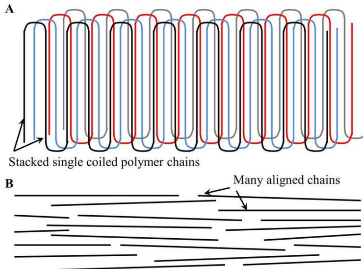
**FIG. 8:** Illustration of a polymer crystal and aligned polymer. (A) Polymer crystals consist of an array of stacked chains each of which is coiled, forming a #D lattice structure (individual molecules are shown with different colors). (B) Aligned polymers consist of an array of chains that are straightened with a high degree of axial alignment.
