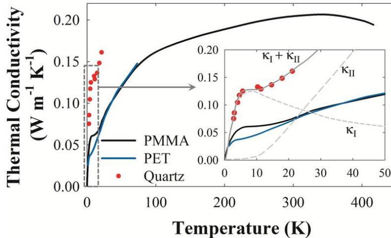
**FIG. 4:** Thermal conductivity of quartz, amorphous polymethyl methacrylate (PMMA) and polyethylene terephthalate (PET). Inset shows the low-temperature behavior and transition between the dominant contribution from normal and Umklapp phonon scattering. The amorphous polymers show similar behavior to that of quartz glass.
