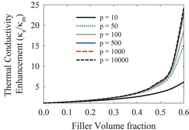
**FIG. 7:** Theoretical prediction of the relative thermal conductivity enhancement for composites ( $\kappa_e/\kappa_m$ ). The ratio of the filler thermal conductivity ( $\kappa_f$ ) to that of the matrix ( $\kappa_m$ ) is given by  $p = \kappa_f/\kappa_m$ .
