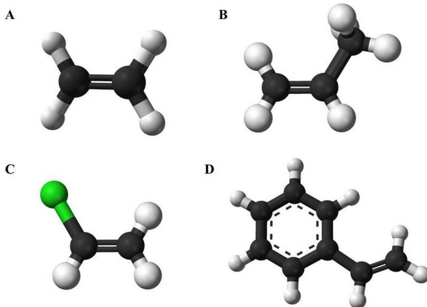
**FIG. 1:** Four of the most commonly produced monomers: (A) ethylene ( $\text{C}_2\text{H}_4$ ); (B) propylene ( $\text{C}_3\text{H}_6$ ); (C) vinyl chloride ( $\text{C}_2\text{H}_3\text{Cl}$ ); (D) styrene  $\text{C}_8\text{H}_8$ .
