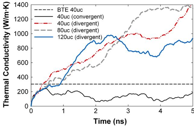
FIG. 2 (color online). Green-Kubo thermal conductivity integrals for different simulation domain sizes. One convergent and one divergent case are shown for the 40 uc simulations, as well as divergent cases for the 80 and 120 uc simulations. The BTE 40 uc line indicates the thermal conductivity computed from the BTE-TC expression, when contributions from the two non-attenuating modes are neglected.
