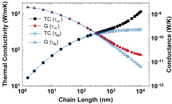
FIG. 4 (color online). Thermal conductivity (circles) and corresponding thermal conductance (triangles) predictions for a single PE chain. The  $\tau_\infty$  curves assume that the (potentially nonattenuating) modes of polarizations 1 and 4, with wavelengths larger than 40 ucs, have infinite phonon-phonon relaxation times. The  $\tau_{\text{fit}}$  curves use extrapolated values for the relaxation times of these modes.
